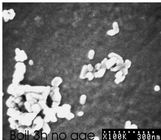
Figure 5 FESEM micrograph of HA nanoparticles produced by the metathesis method.
