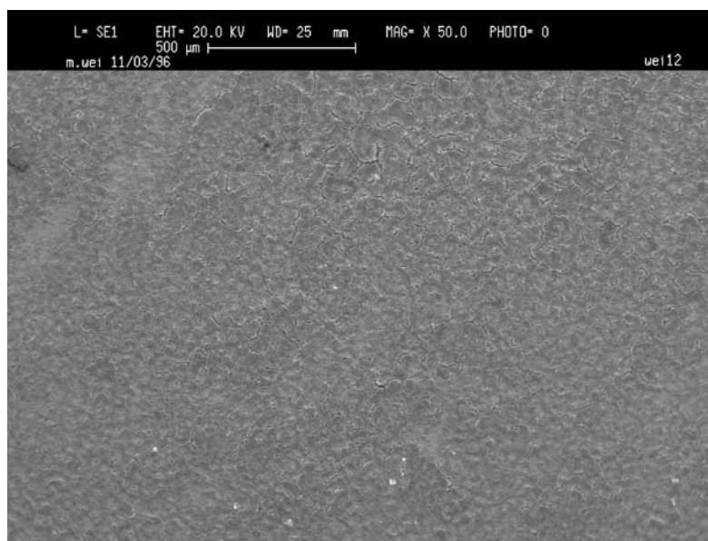
Figure 7 SEM micrograph of the electrophoretic coating produced with calcium acetate HA.
